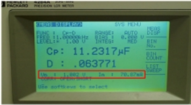
Fig. 2: Voltage and Current level monitors on the HP4284A.
